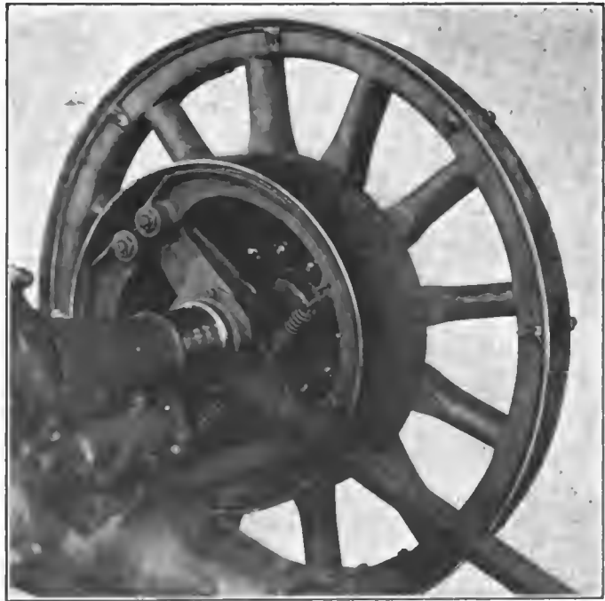
Fig. 4—Rear brake drum, wheel, and details of holding brake mechanism
